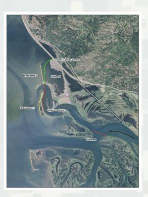
Lower C string booms contain drift in the driftyard (drift holding facility). Drift floats in the facility at summer pool, and is grounded when the area is dewatered in winter.
